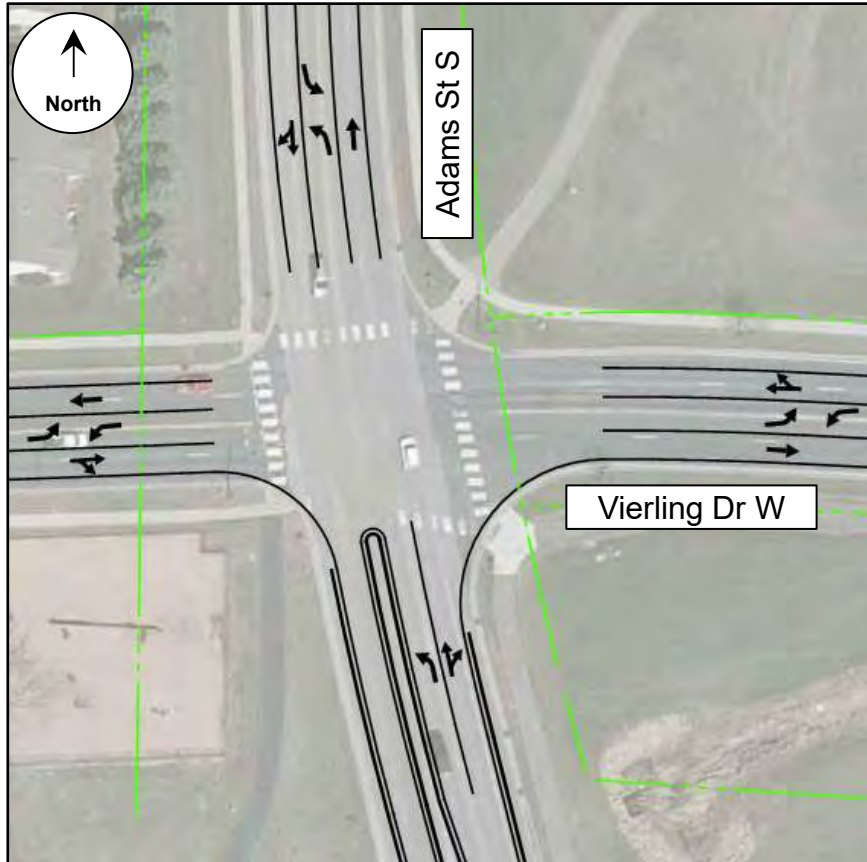
All-Way Stop and Traffic Signal Alternatives
